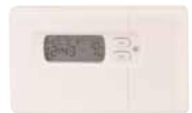
Digital programmable, automatic changeover thermostat with single stage compatibility. Can be used on any zone of an Ultra-Zone control panel. The EWT-AC requires 3 wires R-Y-W and optional G for independent fan control from any zone. Not for use on "ST" panels. **List \$299.00**
