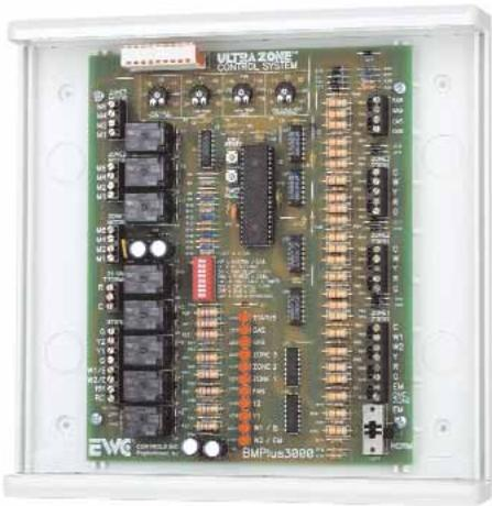
The BMPlus control panel is a single stage, two stage, dual fuel, and heat pump compatible panel controlling up to seven zones. The system features automatic changeover and fan control from any zone with a built in computer “watchdog circuit” to insure proper operation. The BMPlus is supplied with an SAS sensor for high and low temperature limit control that has field adjustable temperature limits.
